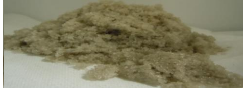
Figure 4.20: The picture at top is of sand for Rhodia A after a foam flood with no oil present. Bottom picture qualitatively demonstrates the appearance of sand after the foam flood displacing crude oil. Rhodia A seems to be poorly swept compared to all surfactant solutions. Rhodia B foam has taken many PVs but the sand appeared to be entirely clean. AOS foam which had the best overall performance seemed to have left behind some oil. Both the blends had not swept the sand pack clean, with A:AOS 1:9 being the better among the two..
