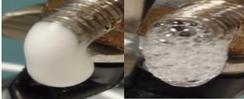
Figure 4.11: Picture of foam at effluent. Left: Transition foam quality (~ 60%) Right: Foam at the high quality regime (~75%-90%). Picture was taken for Rhodia A foam.
