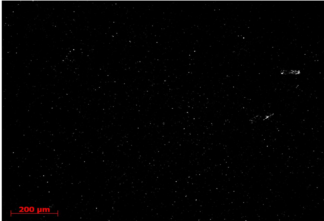
Figure 3.11: Birefringence in sample of Rhodia B (0.3 wt%) in DI water on a 7 day old sample. Image obtained under a cross polarized microscope.
