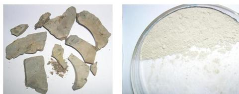
Figure 9 Sample from a carbonate reservoir before and after treated in the shaker box.
