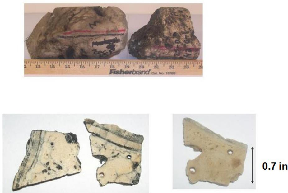
**Fig. 11** sample before trimming (upper image), before cleaning after being cut (bottom left), and after the cleaning process (bottom right). Sample was dissolved in between 10% to 50% excess (assuming dolomite) of hydrochloric acid (1 N), and analyzed via ICP after dilution 1/1000 in aqueous solution at 2% in  $\text{HNO}_3$
