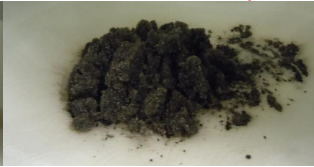
Sand after foam displaces oil
