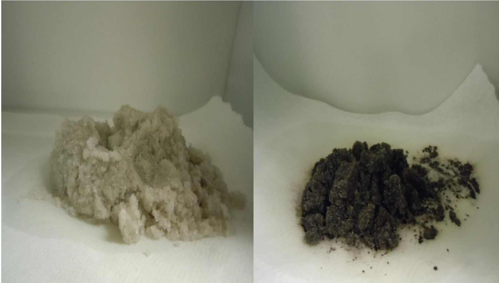
Sand after foamed in the absence of oil
