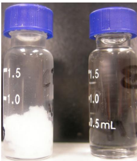
Figure 3-16 0.2% (wt) CTAB in 1% (wt) \text{Na}_2\text{CO}_3 solution. Left one was aged at 125 °C for 11 days, right one was at room temperature
