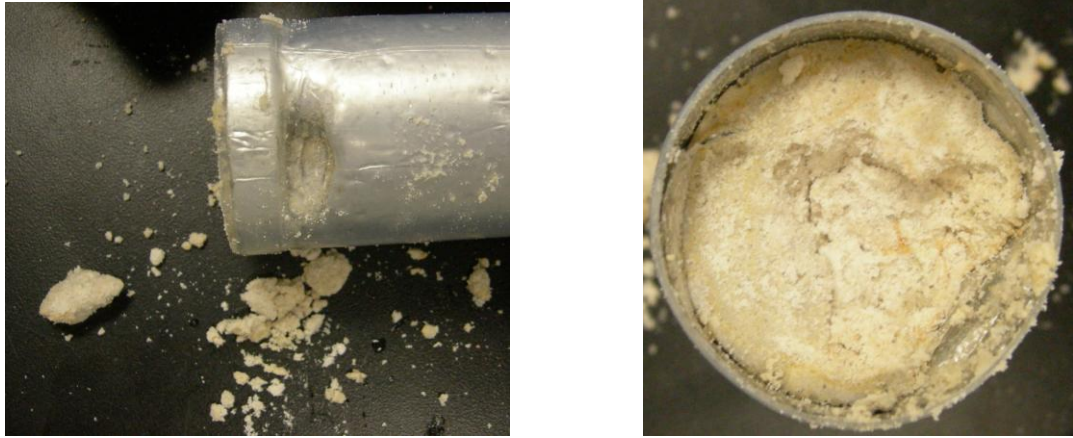
Figure 4-32 The Silurian dolomite core after C12/DI and blend of C12 and CPC in DI water flooding at 120 °C. The solid core was greatly dissolved by surfactant solution in DI water
