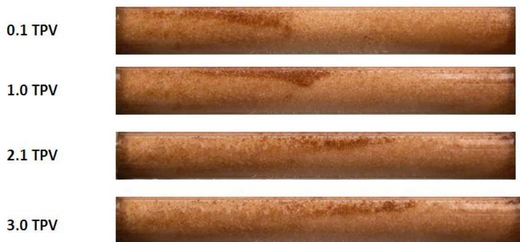
Figure 3-32 The photos for sandpack in AOS foam flooding, at 0.1, 1.0, 2.1 and 3.0 total PV (sum of gas and surfactant solution)
