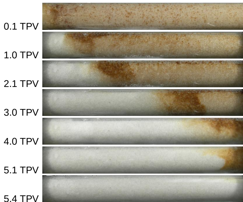
Figure 3-35 The photos of sandpack in AOS-CAB foam flooding, at 0.1, 1.0, 2.1, 3.0, 4.0, 5.1 and 5.4 total PV
