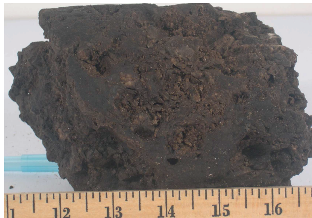
Figure 4.5: Core ID-5; Length = 4.0 inches, Diameter = 4.0 inches; Breccia, very vuggy and heterogeneous
