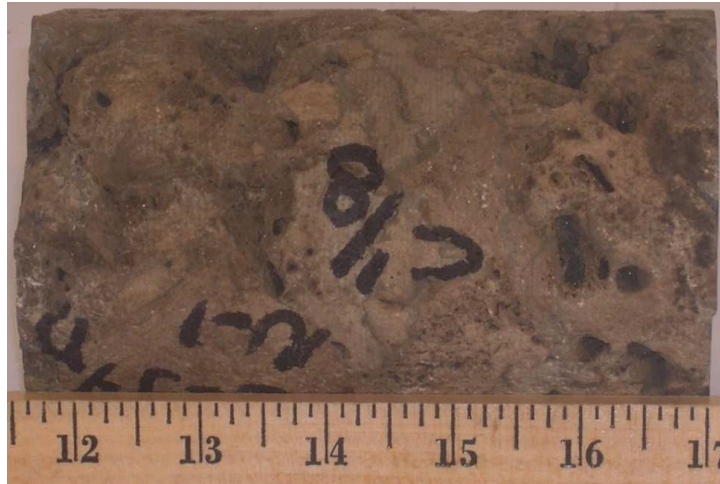
Figure 4.2: Core ID-2; Length = 5.5 inches, Diameter = 3.5 inches; Vuggy, well cored, uniform cylindrical shape
