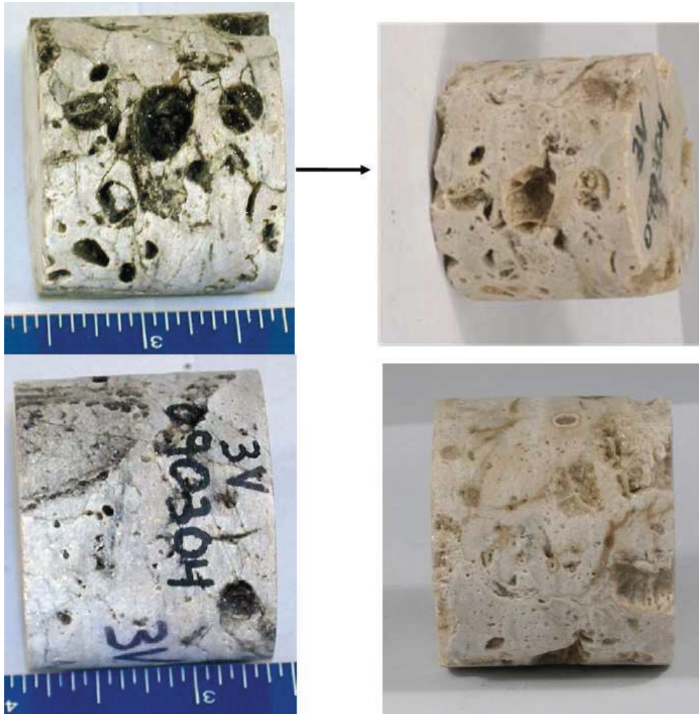
Figure 4.6: A comparison of before (shown at left) and after (shown at right) cleaned pictures for a core-plug (Plug ID: 3V)
