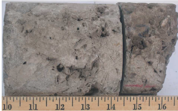
Figure 4.4: Core ID-4; Length = 4 inches, Diameter = 4.0 inches; Some big vugs, well cored
