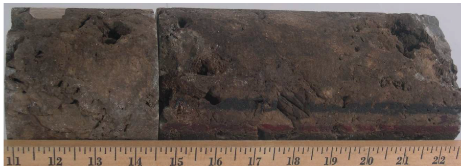
Figure 4.3: Core ID-3; Length = 3.5, 6 inches, Diameter = 3.5 inches; Very vuggy, well cored, uniform cylindrical shape
