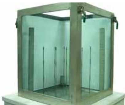
Fig.2 An overlook of the 3-D tank (before sand packing)
